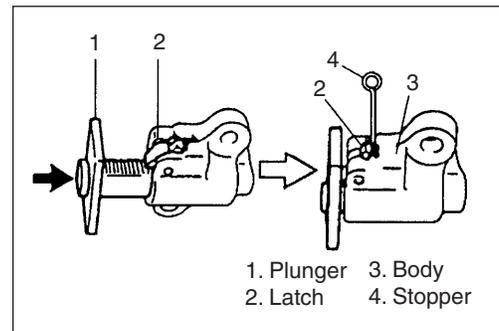
11. Install timing chain tensioner adjuster ⑩.
