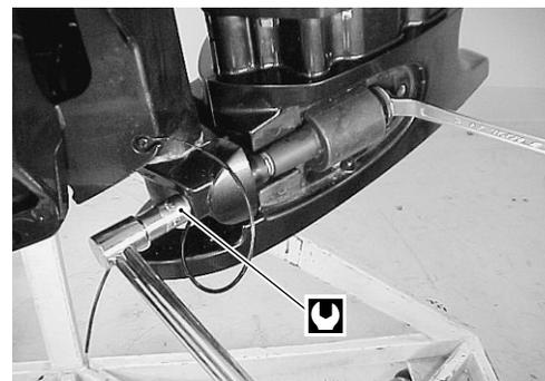
3. Install lower mount covers to driveshaft housing, then tighten lower mount cover bolts securely.
