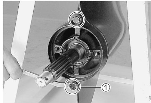
12. Using special tools, draw out propeller shaft bearing housing.
