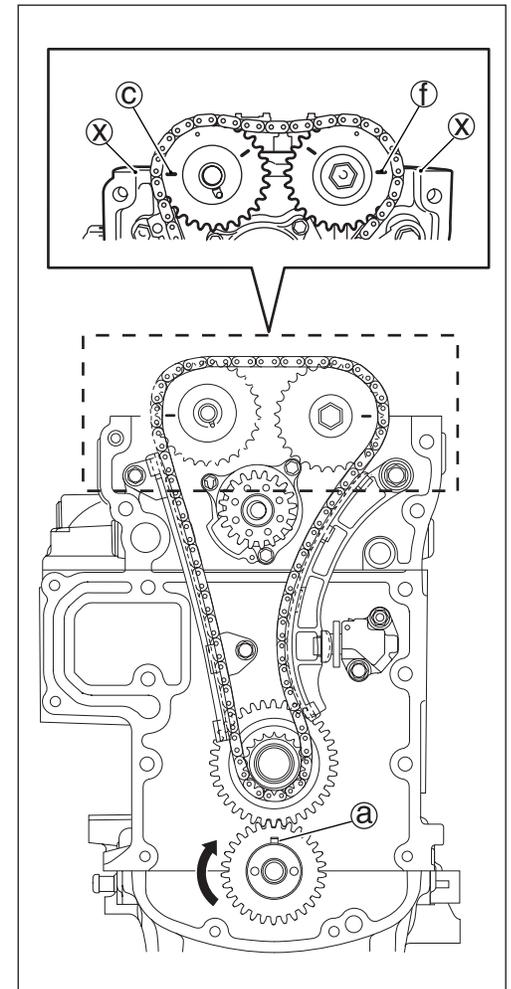
15. Install oil pump drive sprocket ⑪ and tighten bolt securely.
