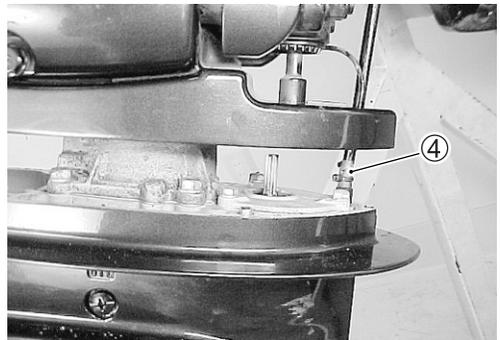
4. Remove clutch rod from clutch shaft (if necessary).
