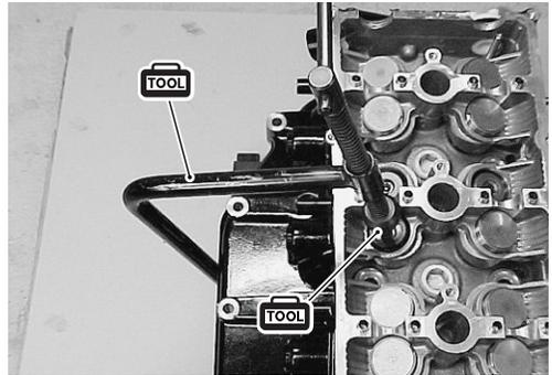
3. Remove valve spring retainer ②, valve spring ③ and valve ④.
