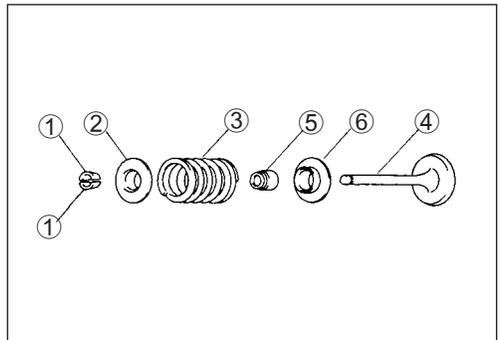
4. Remove valve stem seal ⑤ and valve spring seat ⑥.
