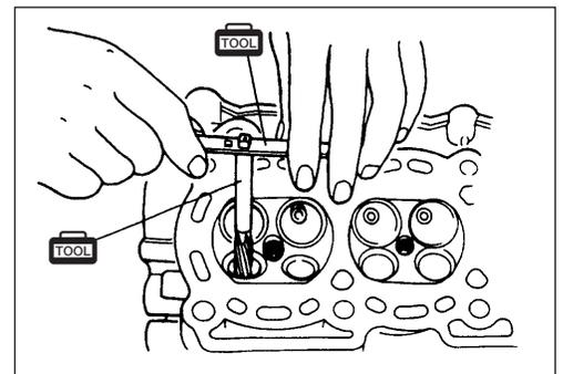
3. Install valve guide to cylinder head as follows.
