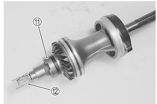
To hold the correct bearing position, pull propeller shaft backward and then install propeller shaft and housing assembly in the gearcase.
