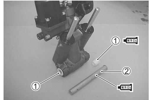
Place the PTT unit in position, then install the clamp bracket. Tighten the clamp bracket shaft nut to specified torque.
