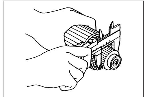
3. Measure commutator undercut (depth) between mica (insulator) and segments.
