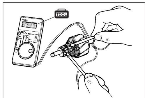
Inspect the commutator surface.
