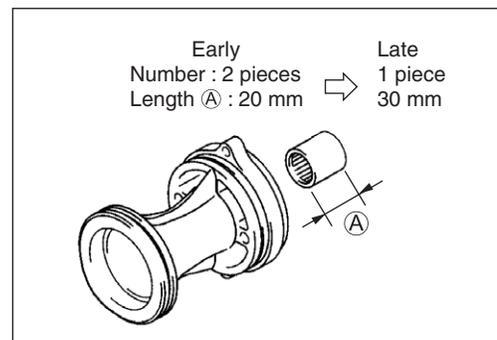
When installing the bearing, stamped mark of bearing must face outside.
