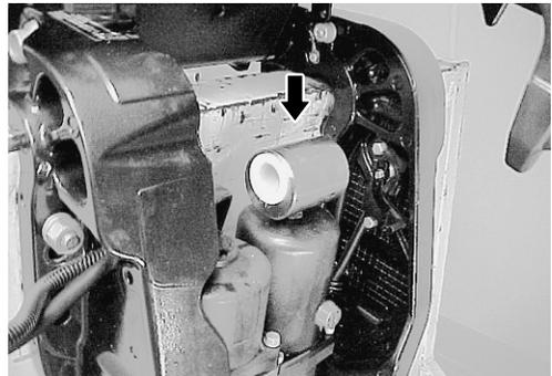
3. Disconnect PTT motor cable wire leads (Green, Blue) from PTT motor relays.
