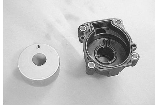
3. Install the pump case No.1 seal into the water pump case.
