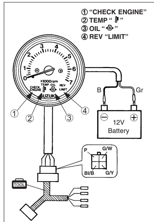
3. Check if lamp lights when connecting battery to test cord terminal as shown.
