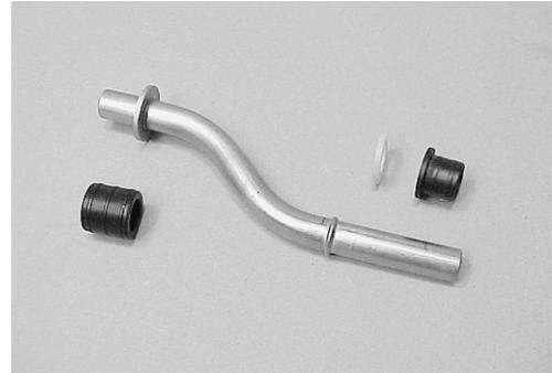
Inspect water tube grommet for excessive wear or other damage.
