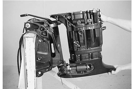
11. Remove two bolts ⑩ and clutch shaft holder ⑪.
