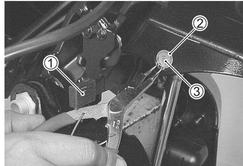
Lower tilt rod to full down position and disconnect the battery cable.
