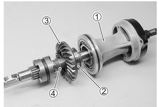
To disassemble propeller shaft components, refer to the following:
