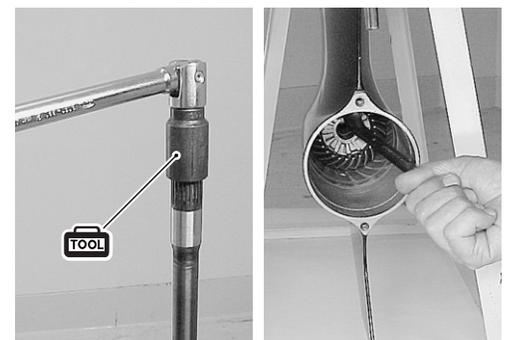
Unscrew the four (4) bolts ① securing driveshaft oil seal housing ②, then remove oil seal housing and pinion shim ③.
