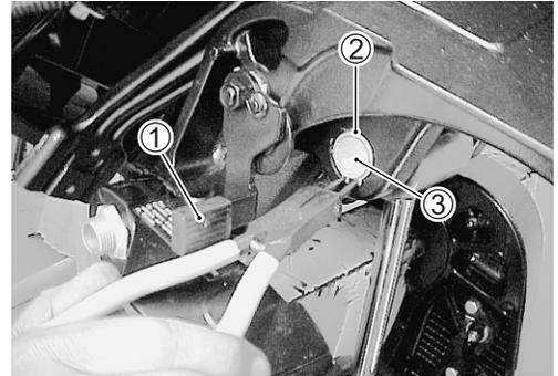
2. Lower tilt rod to full down position and disconnect battery cable.
