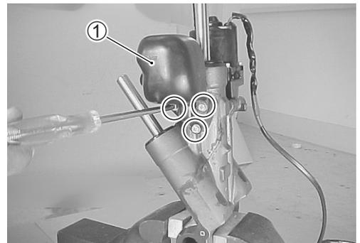
Remove the three (3) screws securing reservoir ①, then detach the reservoir from cylinder body.
