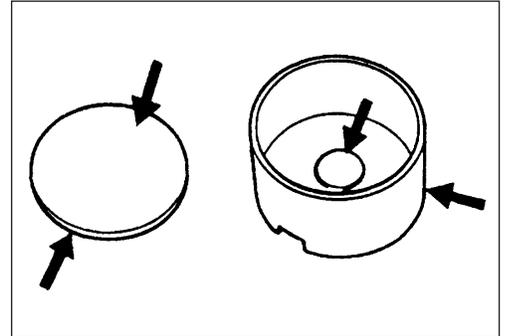
Measure cylinder head bore and tappet outside diameter to determine cylinder head to tappet clearance.
