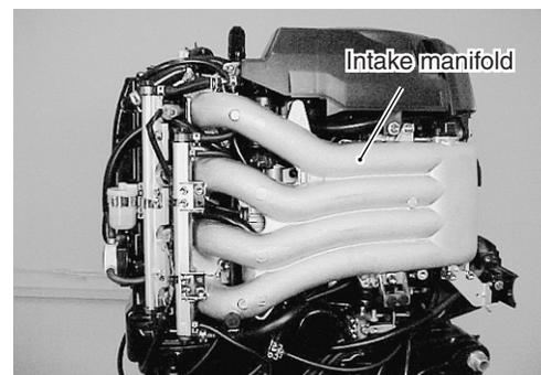
2. Remove three bolts and fuel vapor separator assembly from intake manifold.
