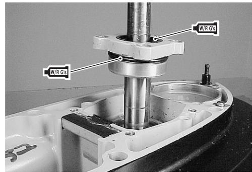
3. Install driveshaft oil seal housing on gearcase, then tighten four bolts securely.
