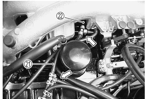
20. Remove nine (9) bolts and two (2) nuts and then remove intake manifold assembly ②③.
