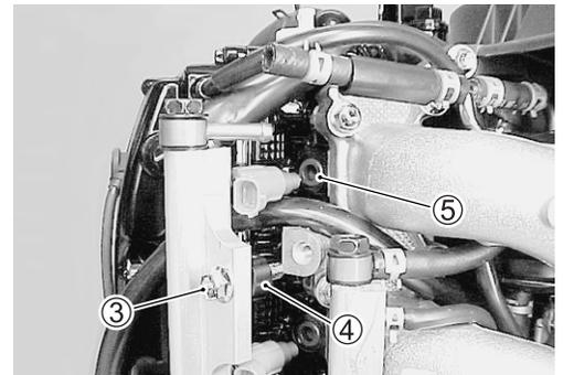
5. Tighten delivery pipe bolt and make sure that injectors rotate smoothly.
