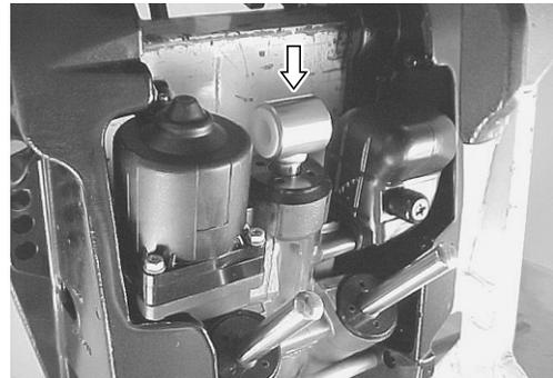
Disconnect the PTT motor cable wire leads (G, BI) from the PTT relays.
