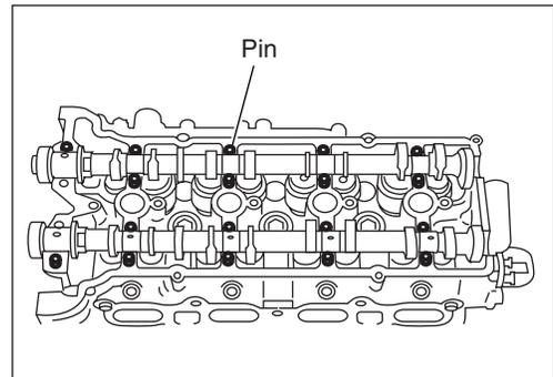
8. Check position of camshaft housing.
