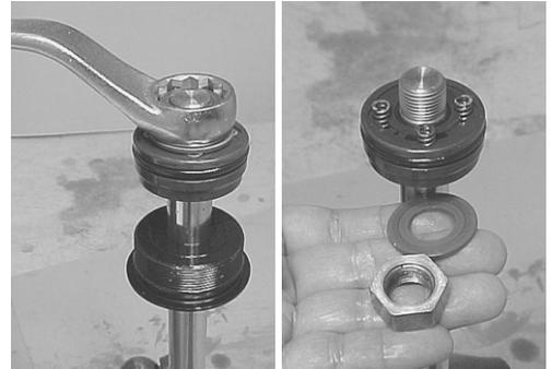
Remove the piston assembly and PTT cylinder head from the tilt rod by sliding them down and off the rod end.
