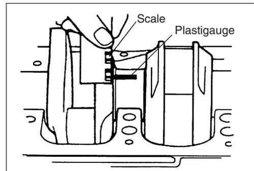
If measurement exceeds service limit, replace crankshaft main bearing.
