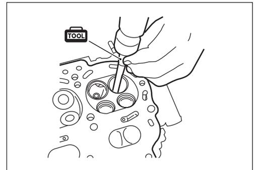
2. Ream valve guide hole with  $\phi 11$  mm reamer to true hole and remove burrs.
