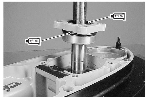
Install driveshaft oil seal housing on gearcase, then tighten four (4) bolts securely.
