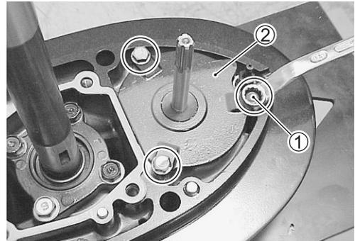
Remove the two (2) bolts ① securing the propeller shaft bearing housing to the gearcase.
