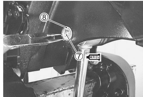
Route the PTT motor cable in through the lower cover and connect the terminals to the PTT relays.
