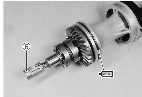
Using special tools, install the propeller shaft and housing assembly in the gear case.
