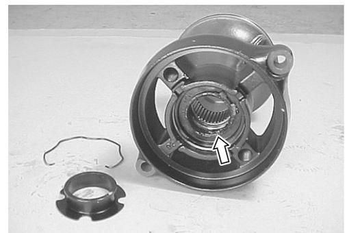
**Replacing propeller shaft oil seal**
