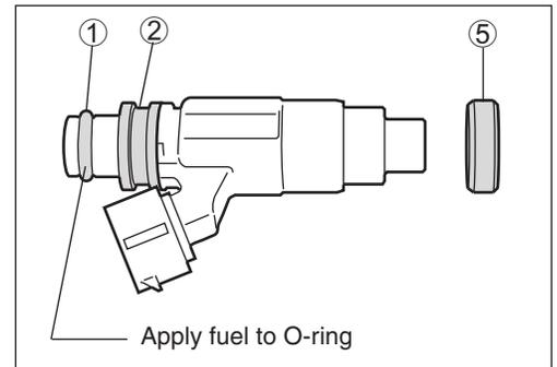
3. Replace injector cushion ⑤ with new one and install it to cylinder head.
