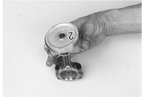
12. Mark cylinder number on conrod using quick dry paint.
