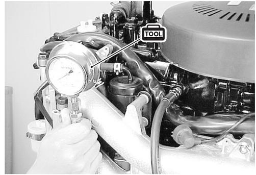
5. Attach engine tachometer to ignition coil high tension cord.
