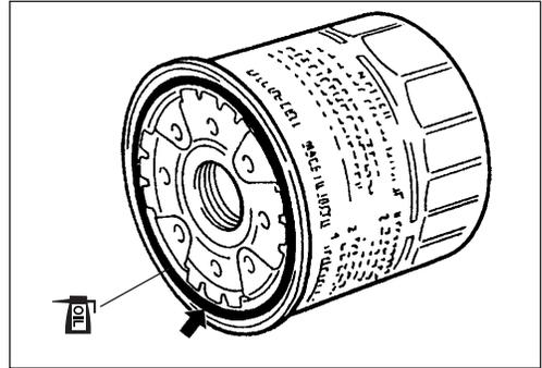
5. Tighten the engine oil filter 3/4 turn from the point of contact with the mounting surface using an oil filter wrench.
