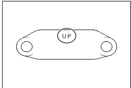
Install the upper mount cover with rib side to be facing to forward.
