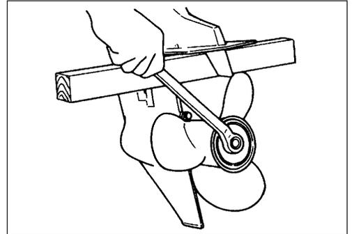
8. Loosen four bolts ①, then remove water pump case ②, impeller ③, impeller key ⑥, pump under plate ④ and dowel pins ⑤.
