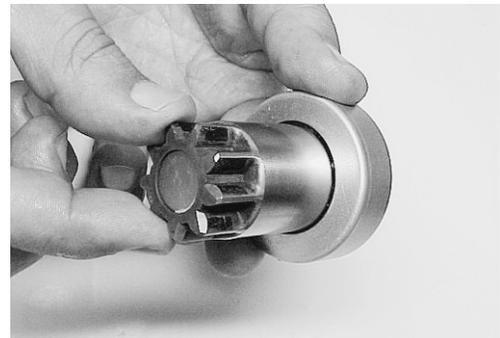
Inspect spline teeth for wear or other damage.
