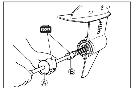
Hold the pinion nut securely, then fit special tool to the driveshaft and loosen the pinion nut.
