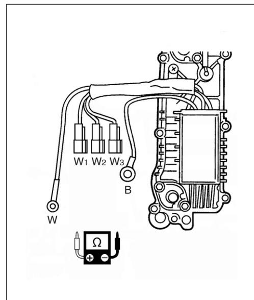
If measurement exceeds specification, replace rectifier & regulator.
