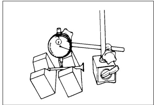
**Valve head radial runout**
