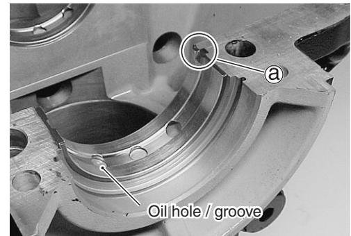
3. Install crankshaft to cylinder.
