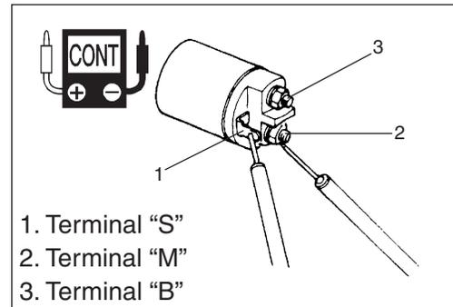
**Hold-in coil Open circuit Test**
