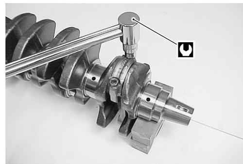
6. Remove conrod and conrod cap from crank pin.
