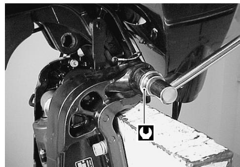
6. Tighten lower shaft bolts ④, pre-coated with thread lock, to specified torque.
