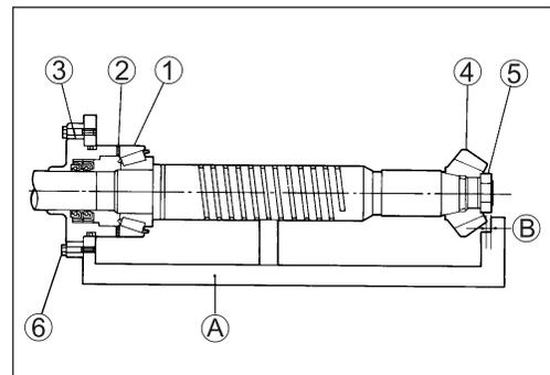
5. Depress and hold driveshaft so that driveshaft bearing is firmly seated in bearing outer race.
