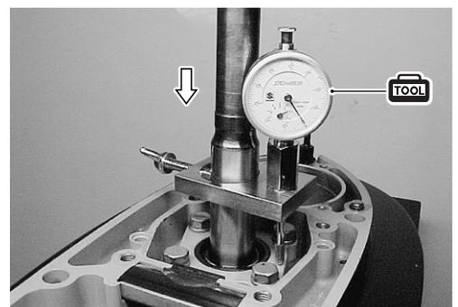
**Checking and adjusting tooth contact pattern
