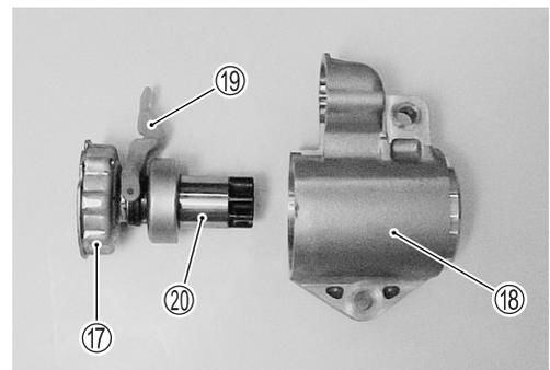
11. Remove shift lever ⑱ and pinion ⑳.
