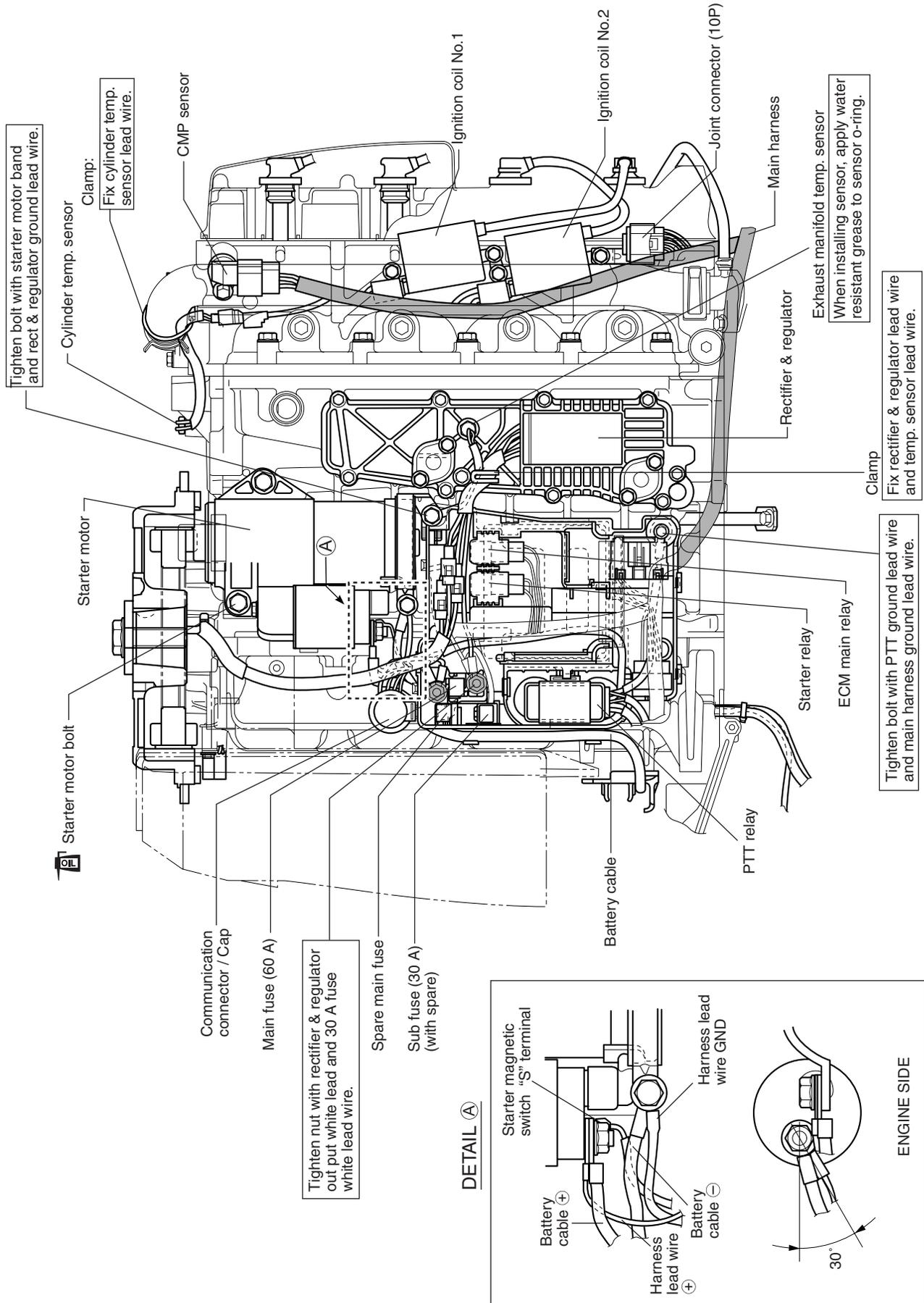
Tighten bolt with starter motor band and rect & regulator ground lead wire.
