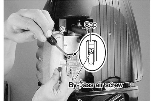
7. When finished adjusting the idle speed, opening the throttle will cancel the (IAC) fixed mode.
