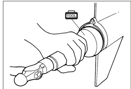
When the housing is fully seated, tighten both retaining bolts to the specified torque.
