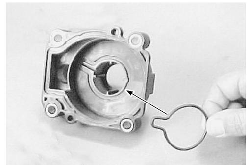
2. Apply Suzuki Bond No.1207B onto the outer-surface of water pump sleeve.
