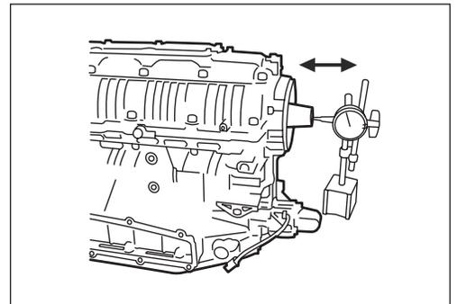
If measurement exceeds service limit, replace crankshaft thrust bearing.
