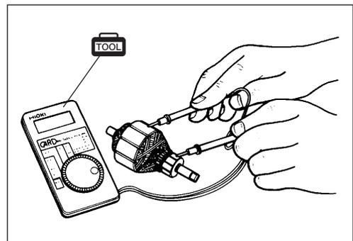
Check continuity between the adjacent commutator segments.
