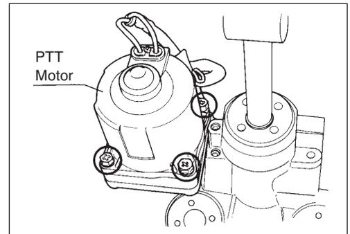
Detach the PTT motor from PTT pump case. Note the position of drive joint ① and O-ring ② and remove them.
