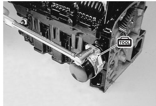
3. Remove oil pressure switch.
