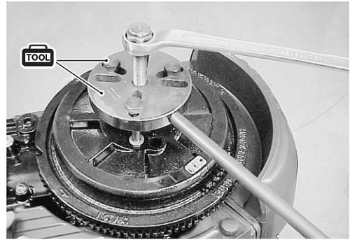
4. Remove flywheel bolt ①, washer ②, flywheel ③ and key ④.
