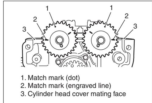
7. Install camshaft housing pins as shown in figure.
