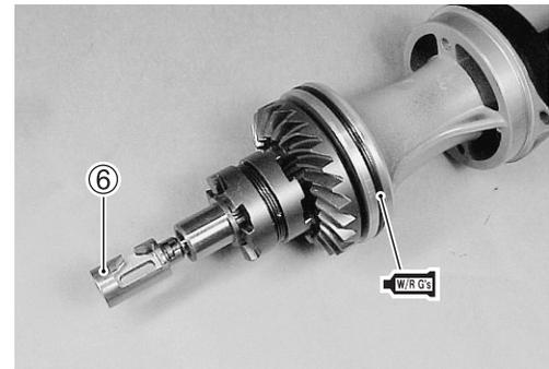
3. Using special tools, install propeller shaft and housing assembly in gear case.
