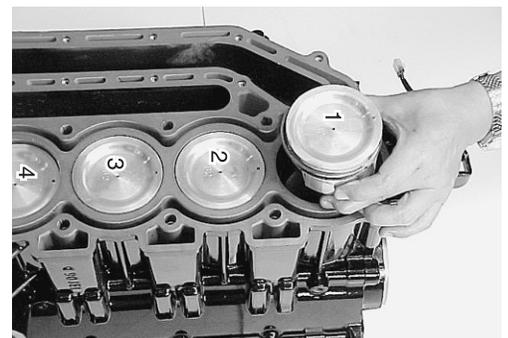
11. Remove two compression rings (top and 2nd) and oil ring from piston.
