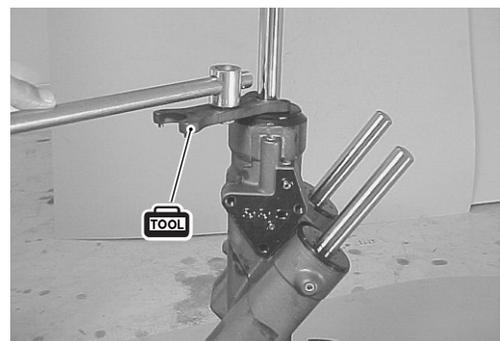
Pull the tilt rod/piston assembly ① out of the cylinder body.
