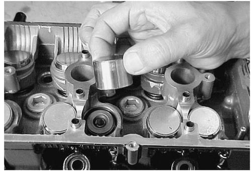
2. Using valve lifter and attachment, remove valve cotters ① while compressing valve spring.
