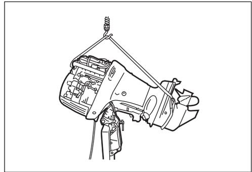
1. Remove tilt rod snap ring ② and push tilt cylinder upper shaft pin ③ out.
