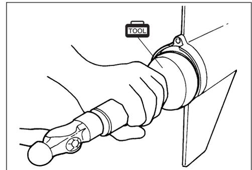
4. When housing is fully seated, tighten two bolts to specified torque.
