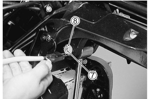
12. Route PTT motor cable in through lower cover and connect terminals to PTT motor relays.
