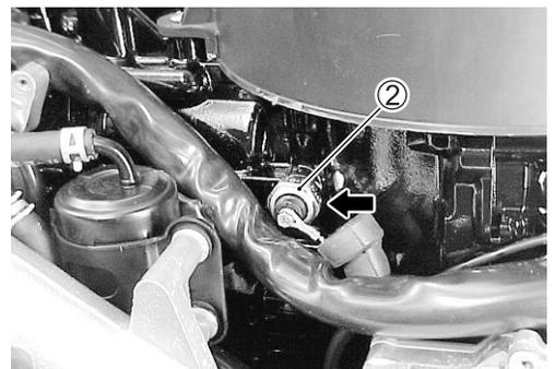
4. Install oil pressure gauge in place of pressure switch hole.
