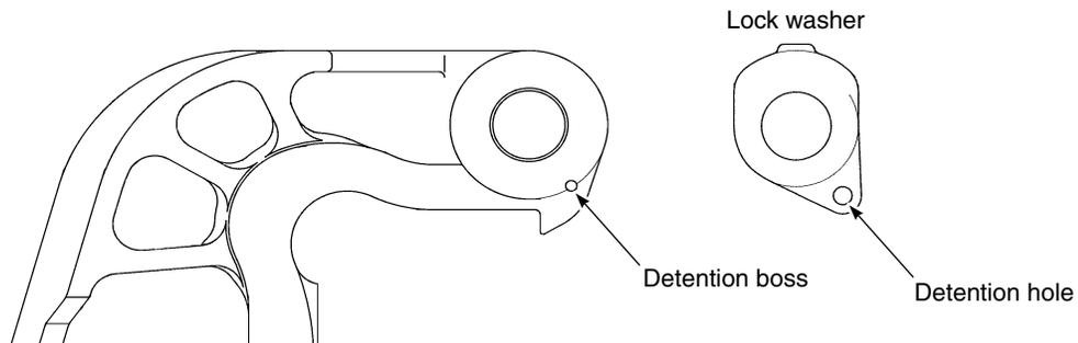
To prevent the lock washer from rotation, a boss has been added to the clamp bracket.
