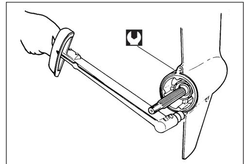
**RECHECKING DRIVESHAFT THRUST PLAY**
