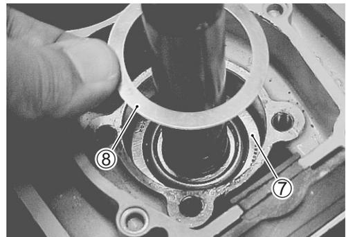
**DRIVESHAFT OIL SEAL HOUSING**
