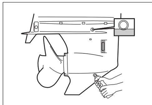
5. Install oil level plug before removing oil filler tube from drain hole.
