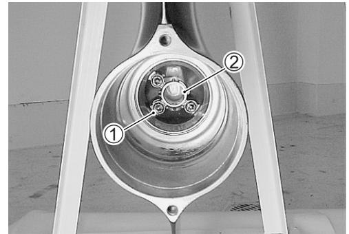
**Disassembly of propeller shaft components**
