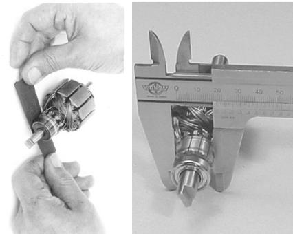
If measurement exceeds service limit, replace armature.
