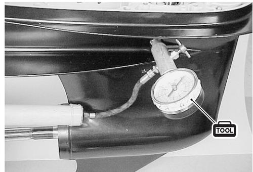
4. Once stabilized, pressure should remain steady for at least 5 min.
