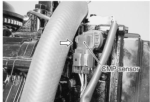
Four trigger vanes are provided on exhaust camshaft and during one rotation of camshaft (two rotations of crankshaft), four high voltage signals are supplied from CMP sensor to ECM.
