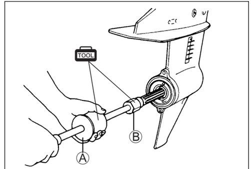
13. Hold pinion nut securely, then fit special tool to the driveshaft and loosen pinion nut.
