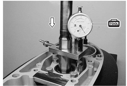
**RECHECKING DRIVESHAFT THRUST PLAY
