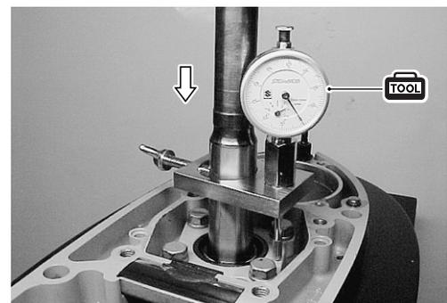
**CHECKING PROPELLER SHAFT THRUST PLAY**
