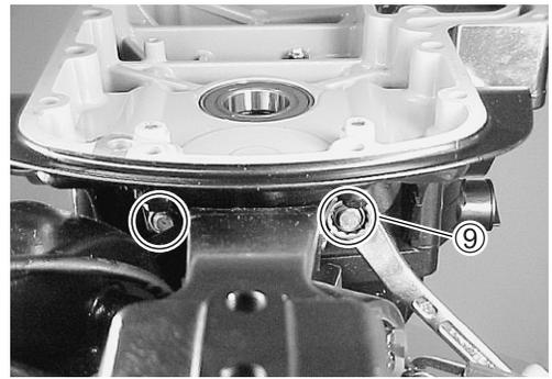
10. Remove driveshaft housing with oil pan.
