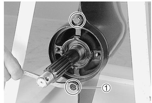
Using special tools, draw out the propeller shaft bearing housing.
