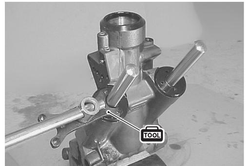
Pull the trim rod/piston assembly out of the trim cylinder.
