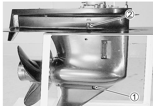
Remove cotter pin ② from propeller nut and remove propeller nut ③.
