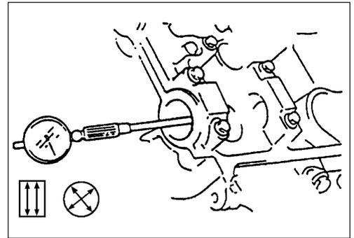
**TAPPET / TAPPET SHIM****Wear of tappet and shim**
