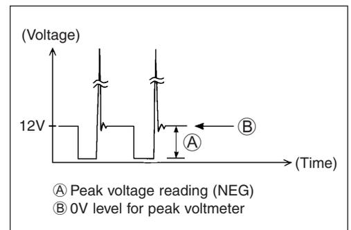
4. Crank engine and measure voltage.
