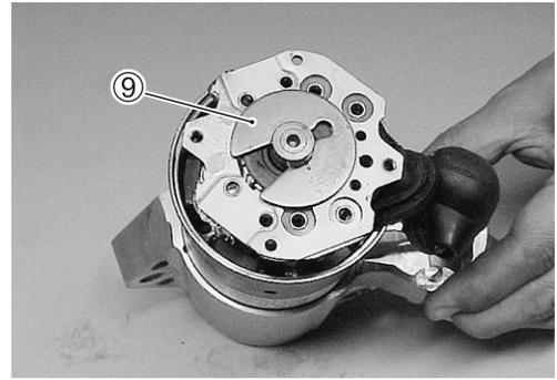
6. Pull brush spring ⑩ up so that brush is separated from surface of commutator, then remove brush holder ⑪.
