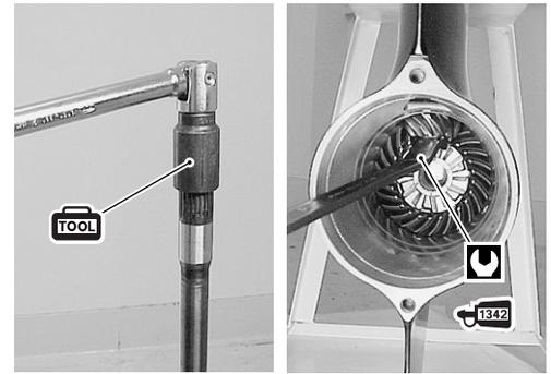
**CHECKING DRIVESHAFT THRUST PLAY**
