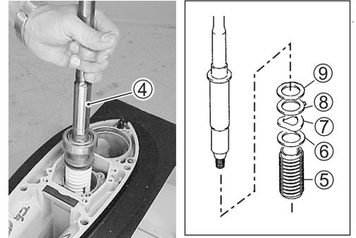
Remove the pinion gear ①.
