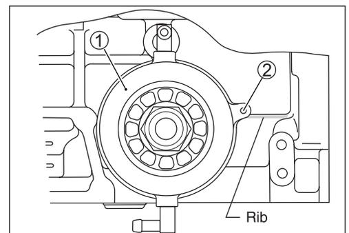
3. Install oil filter stand ③, then tighten filter stand to specified torque.
