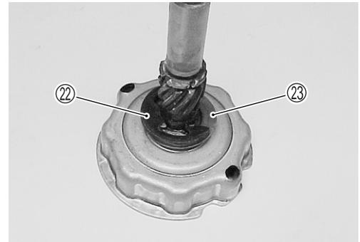
13. Remove pinion shaft ㉑, washer ㉓ and rubber ring ㉔ from center bracket.
