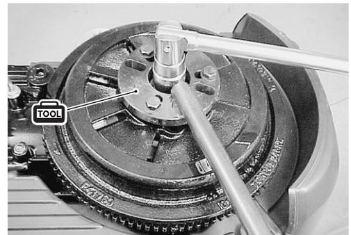
3. Using special tools, loosen flywheel from crankshaft.
