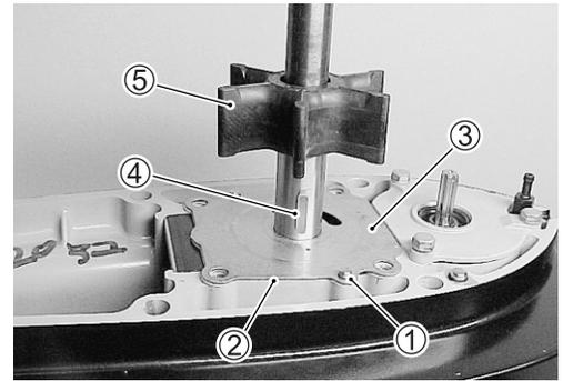
3. Install pump case ⑥ while rotating driveshaft clockwise to flex impeller vanes in correct direction.
