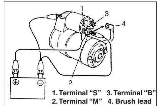
2. While connected as above with plunger out, disconnect negative lead from terminal "M".
