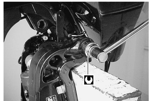
Tighten lower shaft bolts ④, pre-coated with thread lock, to specified torque.
