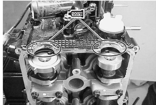
2. Assemble new O-rings and cylinder head cover gasket to cylinder head cover.
