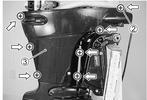
3. Remove two screws ④ and PORT side cover ⑤.
