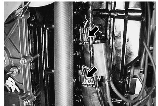
5. Make sure fuel pressure has been removed by pinching high pressure fuel hose with finger tips (line should feel soft without pressure).
