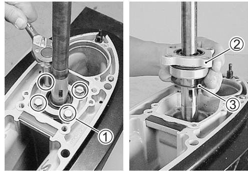
Lift out driveshaft assembly ④.
