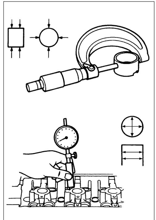
**VALVE / VALVE GUIDE****Valve guide to valve stem clearance**
