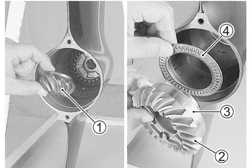
Remove the reverse gear ② from reverse gear retainer ③.
