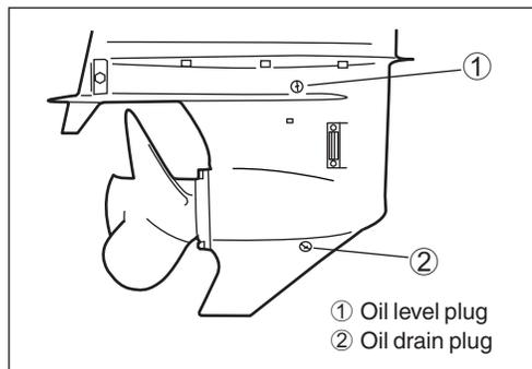
4. Fill with recommended gear oil through oil drain hole until oil just starts to flow out from oil level hole.
