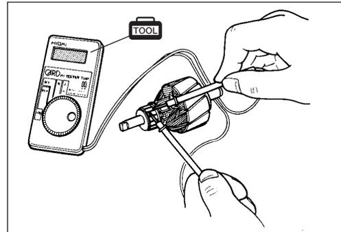
3. Inspect commutator surface for gum or dirt.
