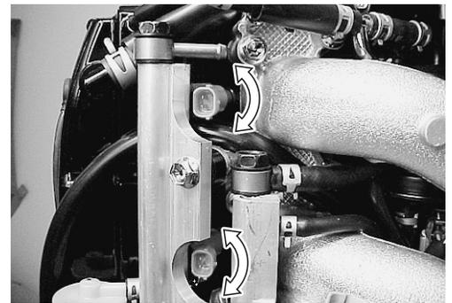
6. Reconnect fuel feed hose to fuel delivery pipe.
