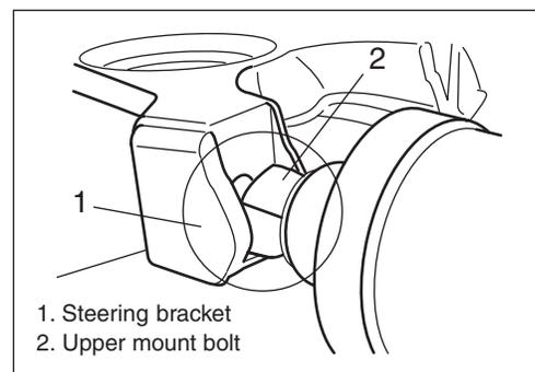
2. Install washer ① and upper mount front nut ②, then tighten two nuts, pre-coated with thread lock, to specified torque.
