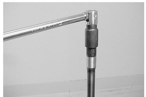
2. Install propeller shaft and housing assembly (minus reverse gear and internal components).
