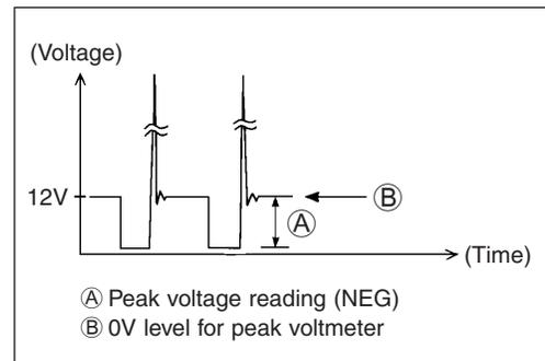
4. Crank engine and measure voltage.
