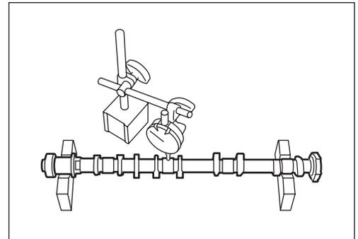
If measurement exceeds service limit, replace camshaft.
