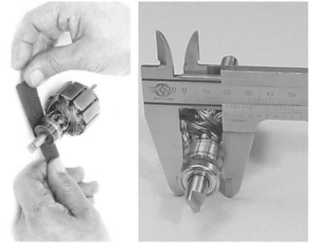
If measurement exceeds service limit, replace armature.
