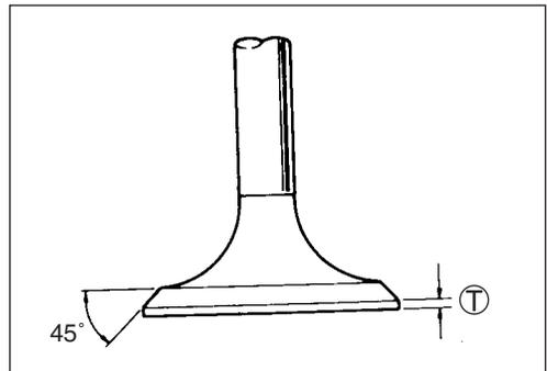
If measurement exceeds service limit, replace valve.
