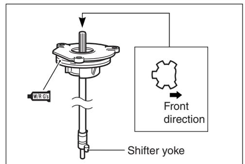
5. Install shift rod guide housing assembly by aligning shifter yoke with groove in horizontal slider, then tighten three housing bolts securely.
