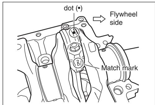
5. Apply engine oil lightly to conrod bolts and tighten nut in two steps.
