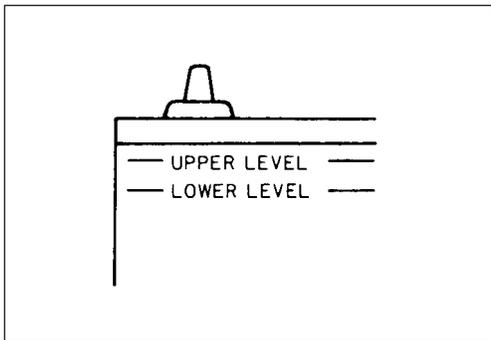
**BATTERY SOLUTION GRAVITY CHECK**
