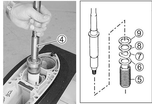
Remove the pinion gear ①.
