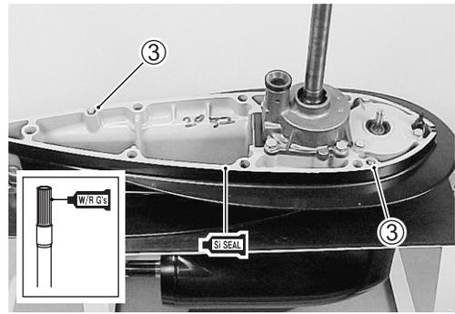
6. Set clutch control lever ④ at neutral position, then slide lower unit ⑤ into place, ensuring that top of driveshaft engages properly with countershaft and that water tube locates in water pump case outlet.
