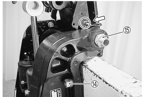
13. Slide STBD clamp bracket ⑯ off clamp bracket shaft, then remove screw and bonding wire from swivel bracket.
