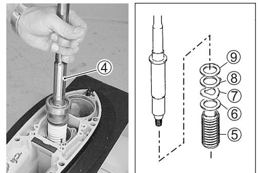
16. Remove pinion gear ①.
