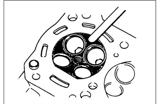
Inspect cylinder head for crack in intake and exhaust ports, combustion chambers and head surface.
