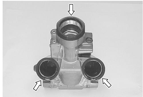
Inspect manual release valve for damage.
