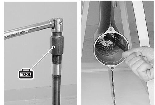
14. Remove four bolts ① securing driveshaft oil seal housing ②, then remove oil seal housing and pinion shim ③.
