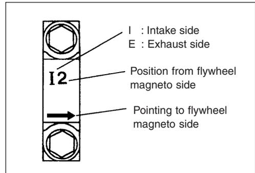
10. Apply engine oil lightly to housing bolts.
