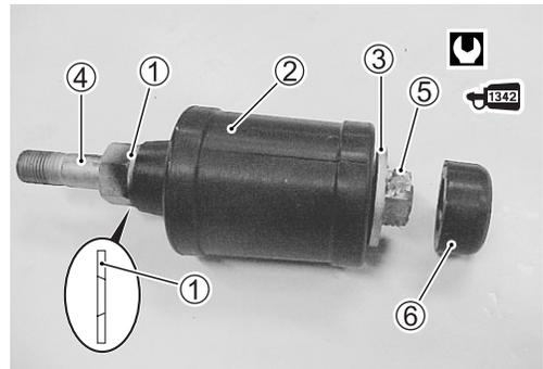
3. Install thrust mount ⑥ to upper mount rear nut, then place upper mount into engine holder.
