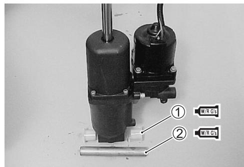
4. Place PTT unit in position, then install clamp bracket.
