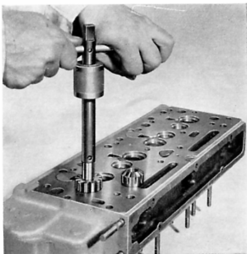
Fig. G.10. Recutting a Valve Seat.
